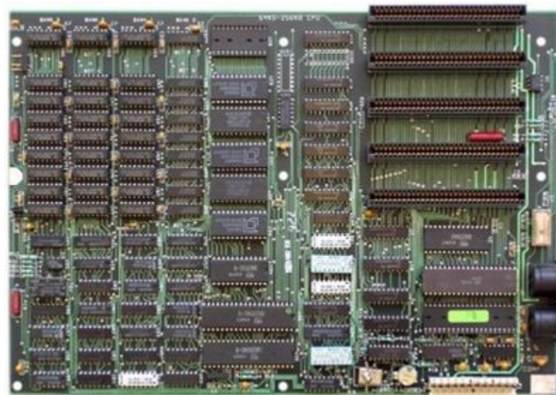
IBM 5150 Personal Computer motherboard. The big chip on the lower right is the 8088. Source: http://gunkies.org/wiki/IBM_5150
